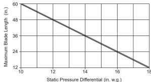
This damper's design at a length of 60" has a maximum allowable blade deflection of L / 360 for the static pressure indicated on the chart. At reduced blade lengths, higher static pressure limits can be attained without sacrificing damper operating performance characteristics.
